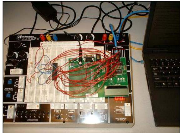
Figure 1. Microcontroller target system and embedded web server interface.
