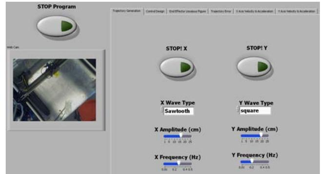
Figure 4. User interface for bi-axial robot control.
